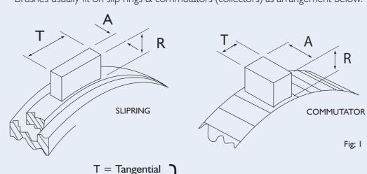
**DIMENSIONS** A = AxialTo the running surface of the collector R = Radial
